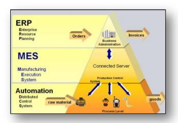
Thus the 'missing' MES sitting at level 2 completes the automation chain, opening up the possibility of developing an **Information Backbone** of the manufacturing enterprise.
